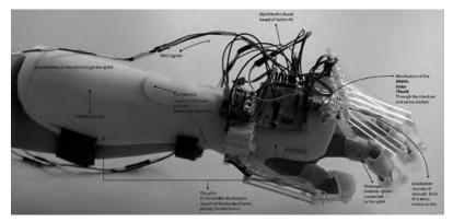
Figure 1: Development from the sketch to the final prototype using traditional and digital prototyping technique to produce MyOrthotics.
