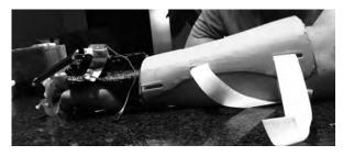
Figure 16. Testing the part and the interaction of the Myoware connection of the Myoware to the SatshaKit and assembling the Satshakit + Myoware + Motor + Orthotics Prototype. https://youtu.be/\_kyQ4P8TT0I
