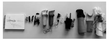
Figure 1: Development from the sketch to the final prototype using traditional and digital prototyping technique to produce MyOrthotics.
