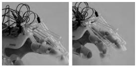
Figure 8 . Extension of the finger through the Exoskeleton and the motors torque (90 degrees). Figure 9. Flexion of the finger through the Exoskeleton and the motors torque (90 degrees)
