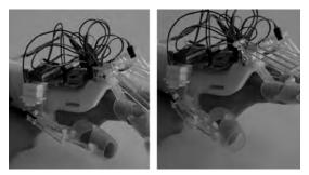
Figure 8, 9. Flexion and extension of the Thumb finger.
